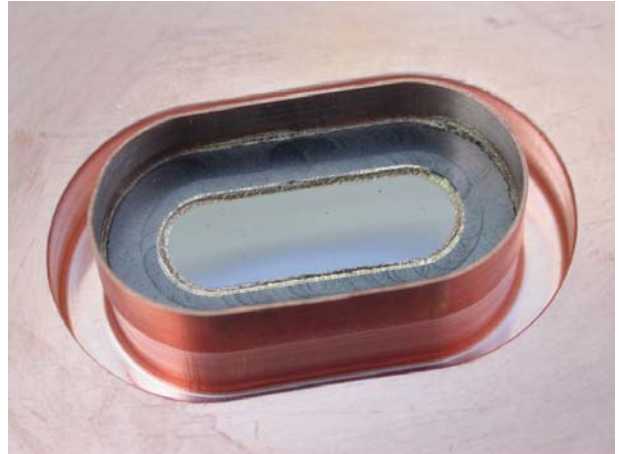
Fig. 7: Detail of the brazing of the CVD foil to the OFHC Cu frame
